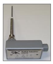
The Model 201LP is powered by an external 24V dc supply and its continuous 4-20 ma output can be connected directly to a PLC, recorder, or digital readout. Changes in the 4-20 ma output are directly related to changes in the concentration of particulate in the gas stream.
