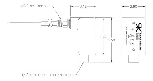
The Model 201LP monitor uses the Triboelectric principle to measure the electrical charge imparted by dust particles as they strike the probe The charge picked up by the probe is converted to an electrical current, which is measured by the electronic system.
